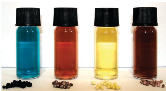
Fig. 6 Photograph of water colloidal solutions of \text{Fe}^{2+}/[\text{Fe}(\text{CN})_6]^{3-} , \text{Cu}^{2+}/[\text{Fe}(\text{CN})_6]^{3-} , \text{Ni}^{2+}/[\text{Fe}(\text{CN})_6]^{3-} and \text{Co}^{2+}/[\text{Fe}(\text{CN})_6]^{3-} NPs and the corresponding chitosan beads (from left to right).
